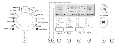
To select a cycle, rotate the Cycle Selector dial to the desired cycle.
