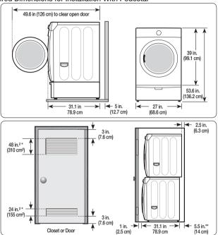
Required Dimensions for Installation With Stacking Kit
